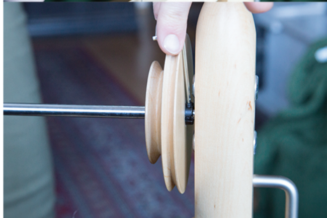
tighten small screw
