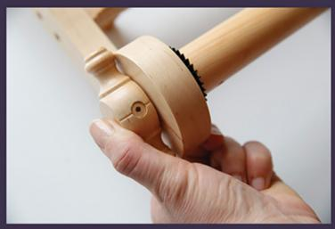
Distance between handle and side should be about 1/24" (1 mm).
