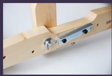
Before screwing the nut add a Small Metal Washer.
