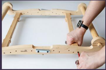
Attach other frame side; place on flat surface and twist frames so all legs are on surface. Tighten all screws
