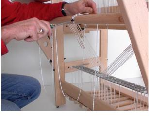
Insert the end of the beater at one side into the nylon bearing of the suspension bar. Be sure that the curve in the beater supports is in the right direction (see picture below).
