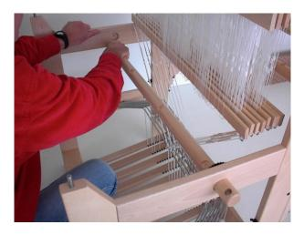
Install the cloth beam in the loom. First insert the side with the ratchet wheel into the hole in the side rail, while you keep the other end of the beam just below the opposite side rail. Because of the beam is slanted in this position, the hole is tight and you have to turn the beam while pushing it through.
