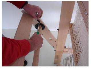
Install a ratchet next to the ratchet wheels of both beams. Use the round head screws 4.5 X 17. Tighten them and then unscrew them just far enough that they can turn freely.
