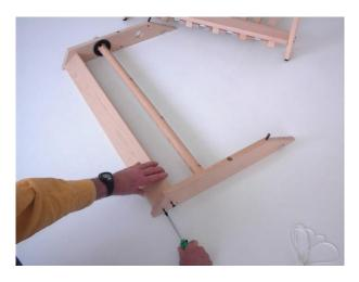
To assemble the back part of the David, use the warp beam supports, the back beam and the warp beam (one of the two round beams with a ratchet wheel).
