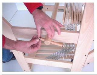
Insert the beam handles through the holes in the beams and secure them by rolling the rubber O-ring into the groove around the handles. The third O-ring in the hardware bag is a spare.
