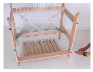
Put the foot rail with the treadles in between the front posts of the loom and connect these parts with the four remaining screws.
