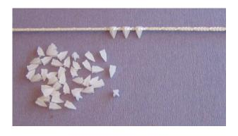
The Texsolv cord is adjustable in length by 12 mm steps (ca.1/2"), according to the loops. For fine adjustment, plastic pegs are used, inserted into the loops of the cord. Each peg through the cord will shorten it about 1.5 mm (1/16"). You will not need more than 7 pegs in a cord, because with 8 pegs the cord becomes one cord loop shorter and you can just as well shorten the cord one loop. In hardware bag 3 are 50 spare pegs.
