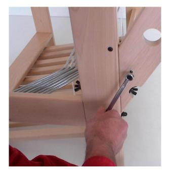
Screw the lag bolt into the warp beam support with wrench number 10 only so far that the thread just disappears in the wood.
