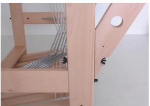
Remove one wing nut and one washer from both threaded ends.
