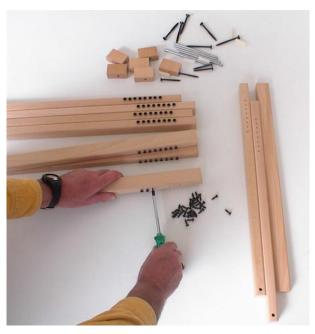
Screw the small screws into the eight holes of each treadle, so far that the screw heads protrude approximately 5 mm (3/16") from the wood. The thread of the screws should just disappear into the wood.
