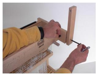
Use the remaining bolts with barrel nut and washer to attach the beater suspension bars at the top of the loom.
