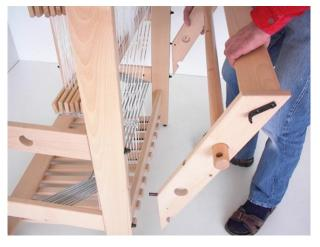
Place the back part in its location by inserting the polyurethane dowels into the holes at the rear of the loom.
