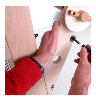
Insert the bolt through the hole in the warp beam support and slip on the large washer.
