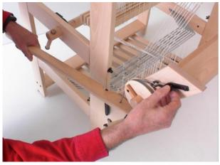
Hook the spring onto the lag bolt and the screw head on the brake handle.
