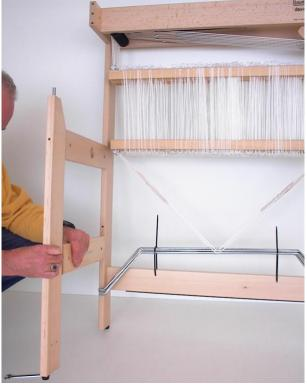
After you mounted all four side rails to the castle section, position the front posts onto the dowels of the side rails.
