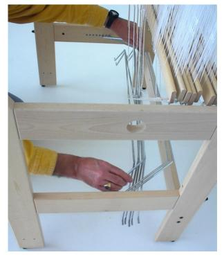
Cut the ties that hold the lams to the back rail.
