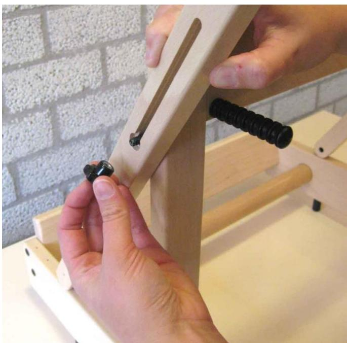
Install the star knobs onto the threaded ends that protrude from the slots in the beater supports.
