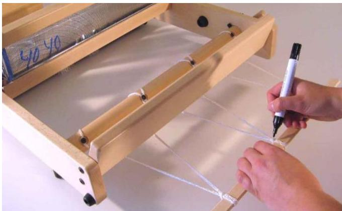
Tighten the half-hitch-loops by pulling on the apron bar.
