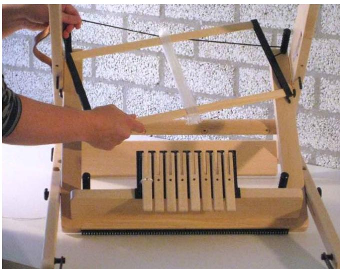
Lead the elastic cord of the shaft over the rollers at the top (normally the bottom) of the loom.
