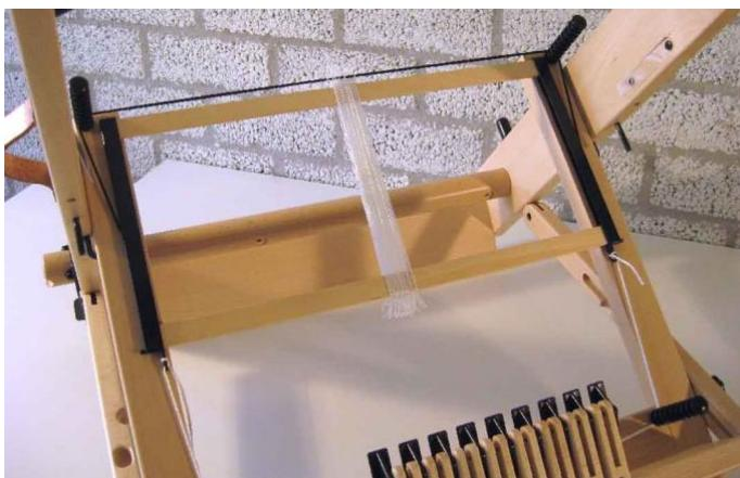
Adjust the position of the shaft as shown in the picture by changing the length of the nylon cord. The distance between the elastic cord and the bottom of the shaft should be about 8 mm (5/16"). You can adjust the shafts more precisely, later on.
