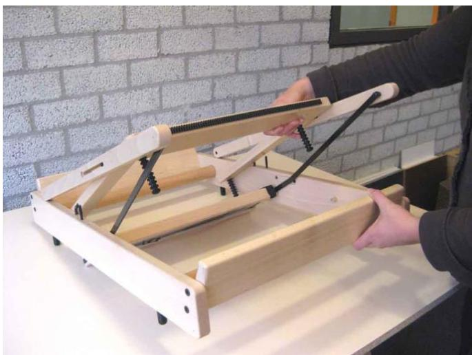
Turn the loom back onto its buffers and unfold it while you lifting the front slightly.
