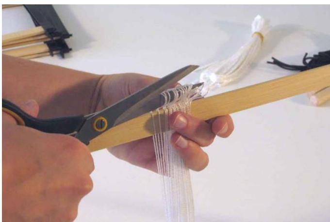
On each shaft, cut the loops that connect the heddles.
