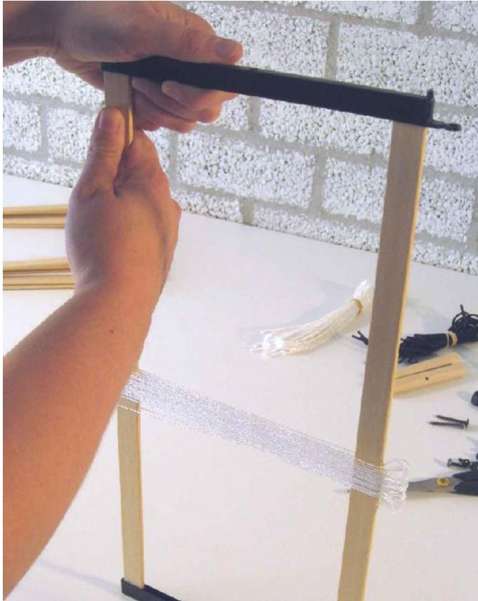
Press the ends of the shaft bars onto the bottom of the shaft sides as shown in the picture.
