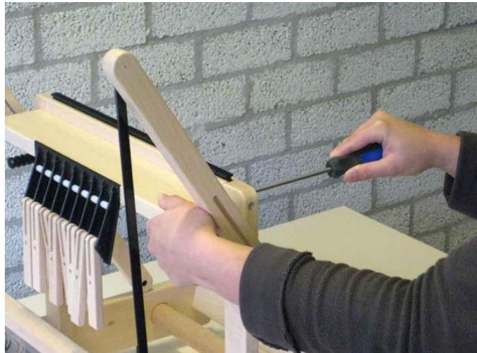
Use the 5 x 50 mm screws to attach the shelf with the toggles onto the loom.
