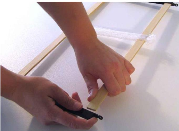
Install the second shaft side and make sure that the eyes at the end of both shaft sides point in the same direction.
