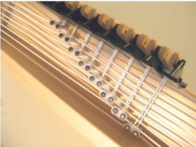
Continue this procedure for each shaft. After you have connected all shafts with their toggles, the cords will form the pattern shown in the picture.
