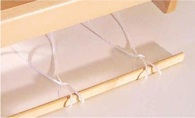
Create a half hitch in the texsolv cord and insert the apron bars, for a total of 3 times.
