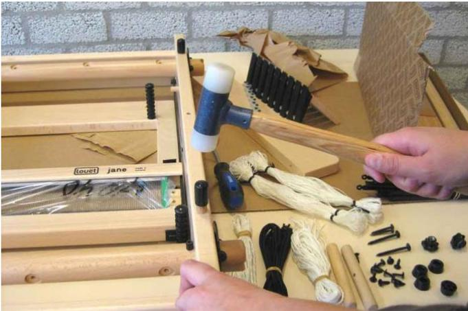
Turn the loom so that the bottom is up, and tap in the four dowels with a rubber coating using a rubber mallet. You will know you have reached the bottom of the holes when the sound changes when hammering.
