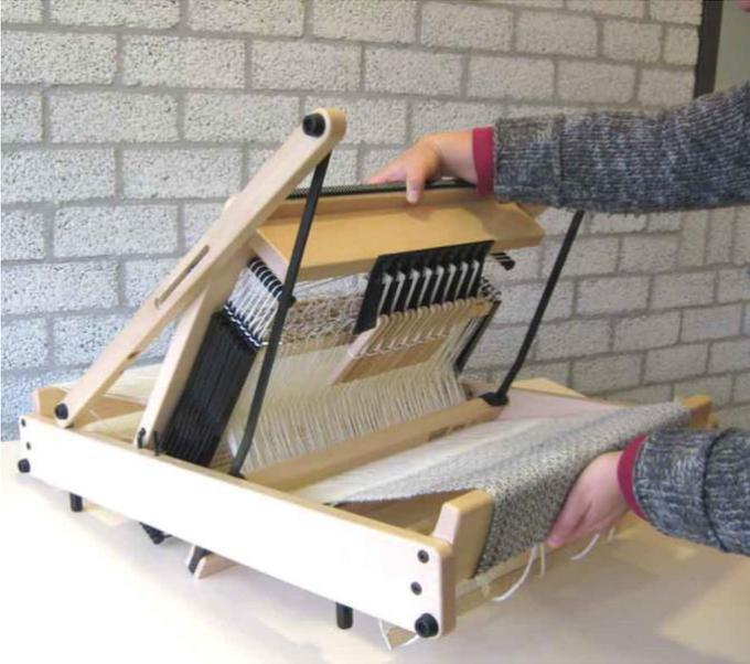
Before you fold the loom again, you have to pull all the toggles down, so all shafts are lifted. If there is a warp on the Jane, you have to release the tension by taking the ratchet out of the ratchet wheel on the cloth beam.
