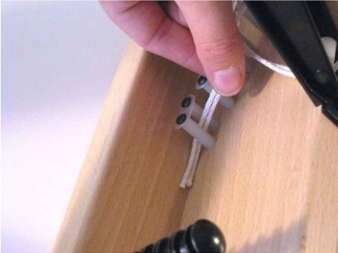
Both ends of the cord have to go between the pair of rollers that line up with the first toggle.
