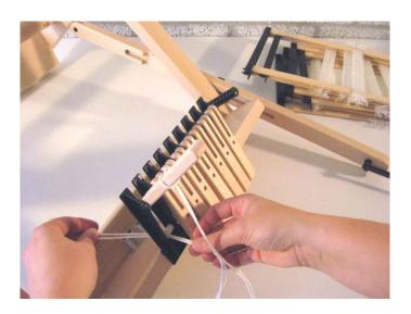
Pull the loop tight and thread both ends of the cord through the opening in between the two toggle hinges and underneath the nylon roller.
