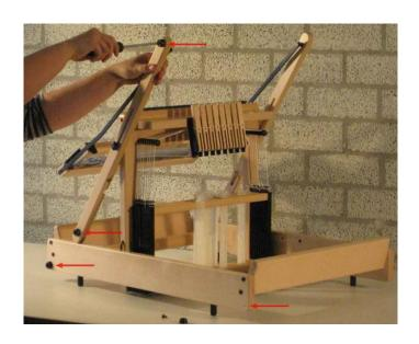
Using the pilot holes, screw the four buffers onto the side of the loom (indicated by red arrows in the picture). When folded, Jane can stand on this side.
