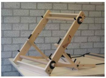
Turn the loom upside down, so that it rests on the back beam and the top of the castle.
