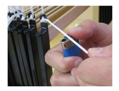
If you want to shorten the ends of the cords, you will need to melt the ends after cutting to avoid unraveling, or cut the cords by melting. Use a lighter or a soldering iron.
