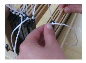
To shorten the cord, pull it while moving the end back and forth as shown on the left picture. The right picture shows how to lengthen the cord; lift the shaft to isolate the cord and use your nail to pull the end of the cord back.
