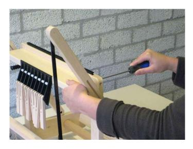
Use the 5 x 50 mm screws to attach the shelf with the toggles onto the loom.
