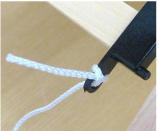
Attach the cord to the eye of the sides of a shaft. Use the knot shown in the picture, created as follows: insert the cord from the inside, where the eye has a sharp edge, and wrap the tail around the notch, tucking the cord so that it crosses on the outside.
