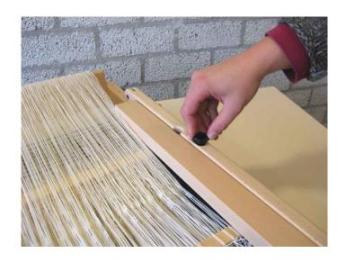
Lock the Jane in its folded position by screwing the black knobs onto the threaded ends located in the hole in the beater supports.
