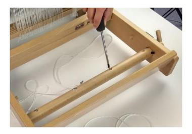
Screw 8 of the 4x15mm screws into the holes of the clothbeam and the warpbeam, so that their heads level with the surface of the beams.
