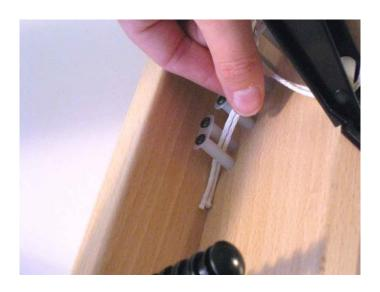
Both ends of the cord have to go between the pair of rollers that line up with the first toggle.
