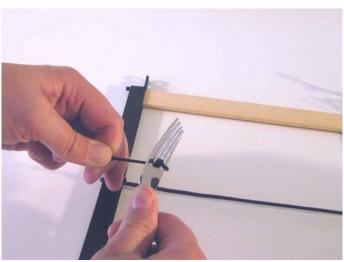
Thread the other end of the cord from the outside through the hole in the other shaft side and make a knot at that end too. Pull the knot into the hollow.
