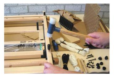
Turn the loom so that the bottom is up, and tap in the four dowels with a rubber coating using a rubber mallet. You will know you have reached the bottom of the holes when the sound changes when hammering.
