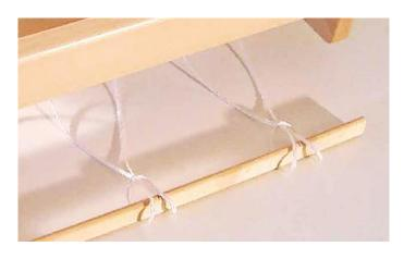
Create a half hitch in the texsolv cord and insert the apron bars, for a total of 3 times.
