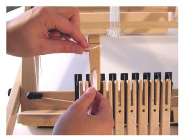
Now, attach a second shaft cord to the next toggle and lead it through in between the hinges and the rollers.
