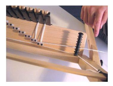
Again, lead the cord ends to both sides, as before. The picture shows how one cord end runs in front of the pair of rollers used by the cord installed previously.
