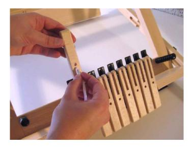
A shaft cord has to be attached to the toggles. Start with the toggle for the eighth shaft; when the loom is in the upside down position shown in the picture, it is the one at the left.
