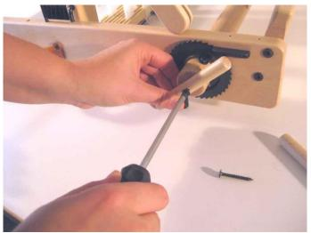
Use the two 4 x 35 mm screws to attach the handles onto the warp and cloth beams.
