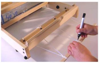
Tighten the half-hitch-loops by pulling on the apron bar.
