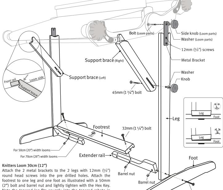
Note the tapered leg fits snuggly into the tapered rebate in the foot. Repeat for the other side. Store the 2 extender rails and  $32\text{mm} (1 \frac{1}{4})$  bolts and barrel nuts for future use with either a 50cm (20") or 70cm (28") Knitters Loom. Proceed to Step 2.
