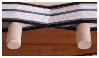
The first cross, between pegs A and B, is the threading cross which keeps the yarn in the correct order for threading. Each thread is separated at the cross.
