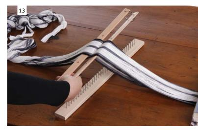
Holding the warp up with the cross sticks place the raddle on the table underneath the raddle cross.
