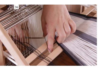
Take the next thread through the eye in the first heddle on the far right of shaft two. Continue working from right to left, taking one thread through the eye in the heddle on shafts three, four, five, six, seven and eight, seven, six, five etc. Continue until all the threads are through the eyes of heddles.
