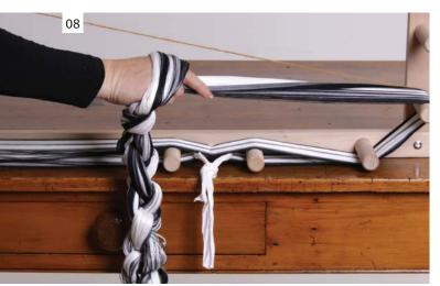
NOTE: For wider warps wind your warp in two or three separate warps. Winding off and chaining each one.
