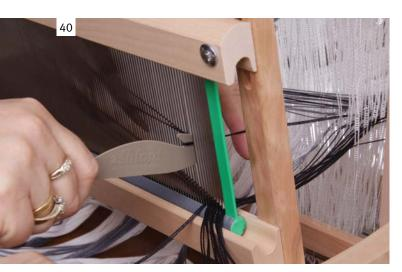
For this project, the sett is 20 epi and there are 10 dents per inch (dpi) in the reed, therefore two ends are placed in each dent. Our project is the full width of the loom, start on the far right slot of the reed. If your project is narrower, take the threads through the slot in line with the outside thread of the warp on the back beam, or measure width from centre of reed.
