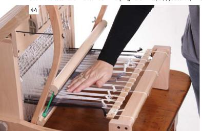
Check that the tension is even across the warp, adjusting the leashing as necessary. Using scrap yarn, weave a heading of plain weave to spread the warp evenly.
