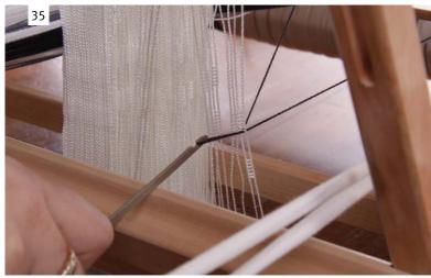
Following the weaving draft from right to left. Take the first thread on the right of the warp, using the heddle hook, pull it through the eye in the first heddle on the far right of shaft one (front).
