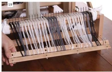
Spread the warp out to the same width as the threads in the raddle. Remove the reed and beater top rail.
