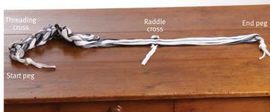
Before you take your warp to the loom you need to prepare the raddle. The raddle will keep the threads spaced correctly as you wind your warp on the loom.
