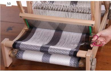
When the weaving is finished cut from the loom. Remove the heading yarn and using a sewing machine, or by hand, hem under ½ in (13mm) at the ends of each towel. Wash in warm, soapy water, dry lying flat and press while still slightly damp.
