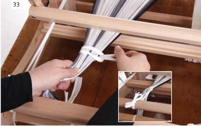
Take the warp through the castle to the left of the heddles. Tie the warp threads with a piece of scrap yarn using a larks head knot. Secure the scrap yarn to the front beam. Remove the tie from the end of the warp and cut the loops.
