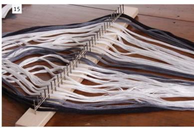
If your project is narrower, count the spaces from the centre pin to ensure the warp is evenly placed on the raddle. The centre pin is marked. Secure the warp with rubber bands.
