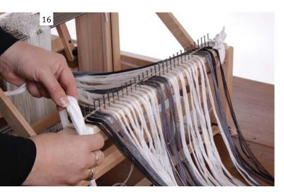
Take the raddle with warp to the loom and secure the raddle to the back beam as shown. Take the beginning of the warp through the castle and let it hang over the front beam.
