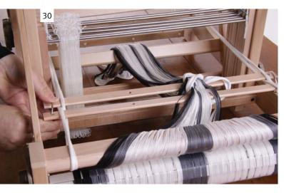
Secure both ends of the cross sticks with the metal rings.
