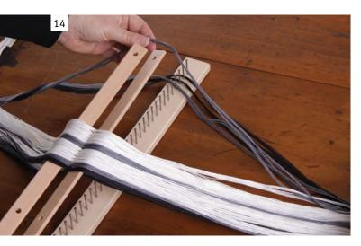
Remove the ring from one end of the cross stick. Slide each group of threads off the cross stick and into the raddle. The raddle used has 32 spaces, and as we have 32 groups we are starting at the end space.
