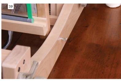
SLEYING THE REED Replace the reed and top rail onto the beater. Hold the beater in place with the cotter pins.
