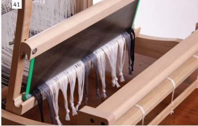
Once sleyed, tie half inch (13mm) groups with a secure knot close to the end.
