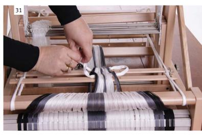
Remove the threading cross tie.
